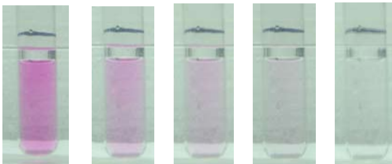
Figure 2: Fading of the phenolphthalein colour with time in a strongly alkaline solution
