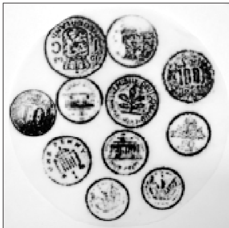
Figure 8. Prints of coins (anode) on filter paper soaked with solution of potassium iodide
