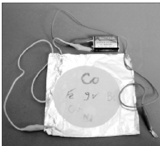
Figure 6. Marks on filter paper soaked with potassium tiocianate, written with Fe, Cu, Ni, Co and Bi anode
